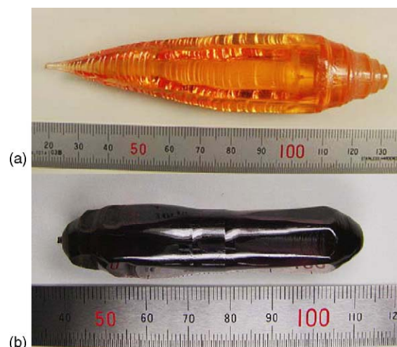
Fig. 1. As-grown (a) \text{La}_3\text{Ga}_5\text{SiO}_{14} , and (b) \text{Nd}_3\text{Ga}_5\text{SiO}_{14} single crystals.
